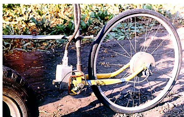
Figure 7. The track wheel mounted on the cleaner
